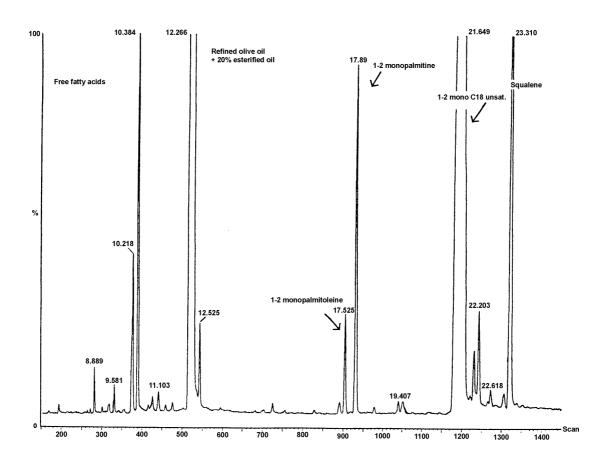
Chromatogram of the silanisation reaction products obtained by lipase action on a refined olive oil spiked with 20% esterified oil (100%).
