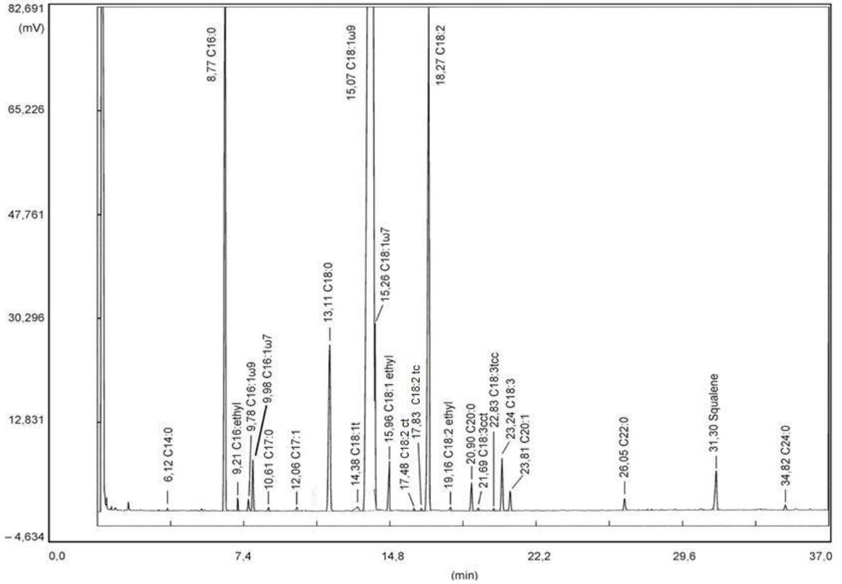
**Figure 1:** Gas chromatographic profile obtained by the cold methylation method from olive-pomace oil. The chromatographic peaks correspond to the methyl and ethyl esters except where otherwise indicated.
