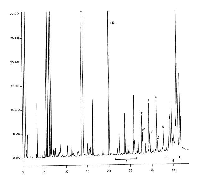
FIGURE: Specimen of a gas chromatogram of the wax fraction of an olive oil (\*)
