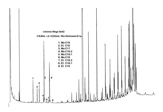
Figure 2 - Chromatogram of virgin olive oil alkyl esters and waxes together
