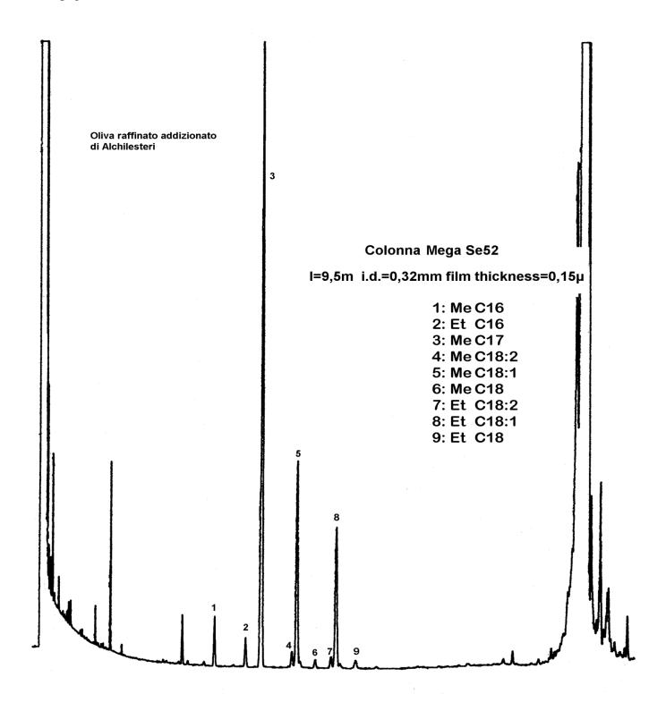
**Figure 1 -** Chromatogram of a refined olive oil spiked with alkyl esters The small peak co-eluted just after Me C18:1 (peak 5) should be integrated with Me C18:1. Same remark for the small peak co-eluted just after EtC18:1 (peak 8)
