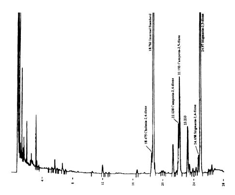
**Figure 2.** Gas chromatographic profile of 1st + 2nd fraction obtained from a mixture of refined olive oil and sunflower desterolised oil on a capillary column (0.25 mm i.d. by 25 m length) coated with 5%-phenylmethylsilicone (0.25 ~m film thickness) using helium as gas carrier.
