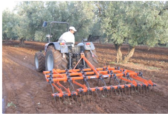
Photo 3: Ploughing with a vibrating tine cultivator
