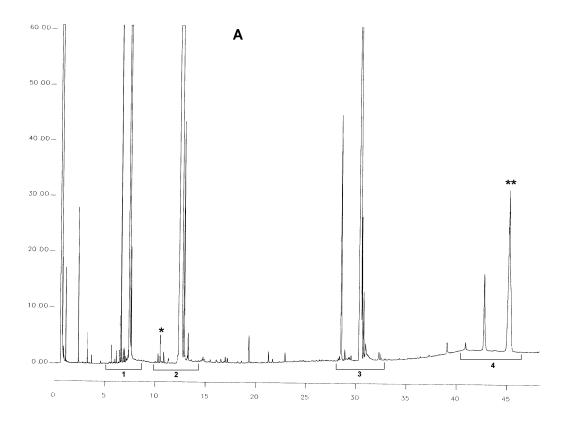
(A) Chromatogram of a genuine olive oil after the action of the lipase, following silanisation. In these conditions (capillary column 8–12 m), the wax fraction elutes with the diacylglycerol fraction or soon after it.
