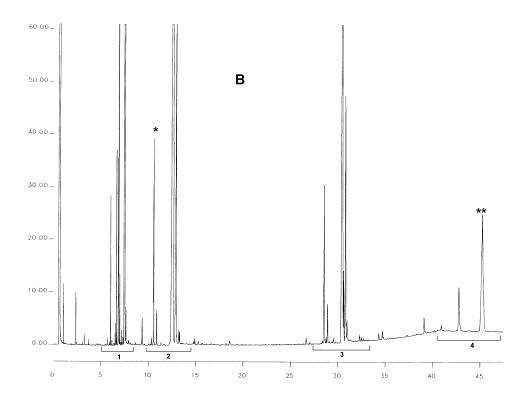
**(B)** Chromatogram of an esterified oil after the action of the lipase, following silanisation. In these conditions (capillary column 8-12 m), the wax fraction elutes with the diacylglycerol fraction or soon after it.
