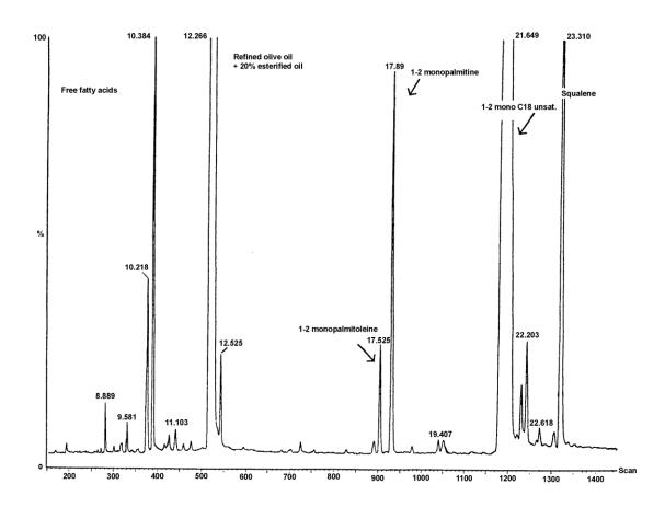
Chromatogram of the silanisation reaction products obtained by lipase action on a refined olive oil spiked with 20% esterified oil (100%).
