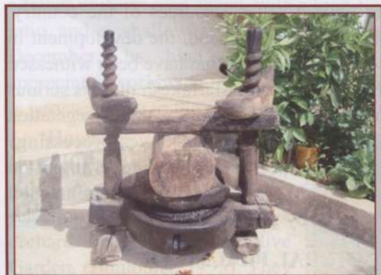
Fig. 10 Home wooden olive press
