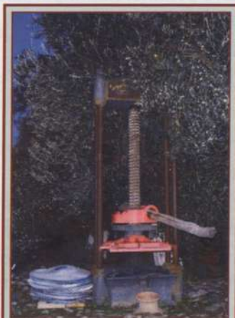
Fig. 4 Hand operated screw press
