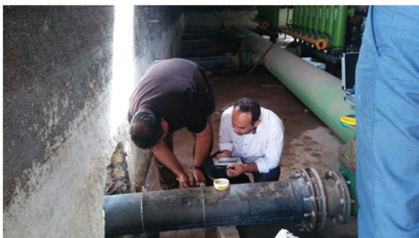
Fig. 1 - Discharge flow monitoring at the entrance of the central control station using an ultrasonic flow meter.
