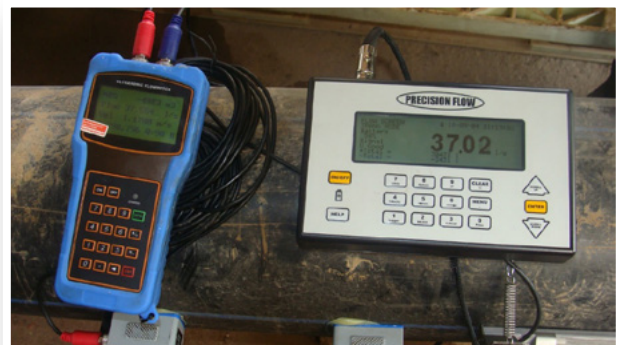
Fig. 2 - Measuring discharge flow at the pumping station using an ultrasonic flow meter (Khandan orchards).
