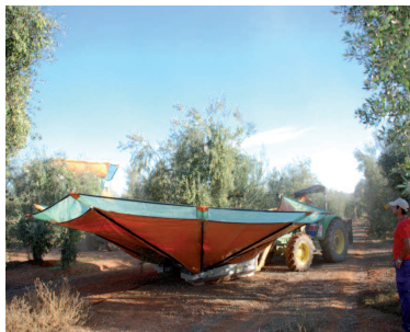
Fig. 3. Inverted umbrella trunk shaker ( left ) and side-by-side trunk shaker ( right ) in intensive olive orchard
