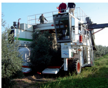
Fig. 4. Straddle harvester for intensive ( left ) and high-density hedgerow ( right ) olive orchards
