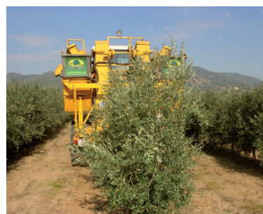
Fig. 4. Straddle harvester for intensive ( left ) and high-density hedgerow ( right ) olive orchards
