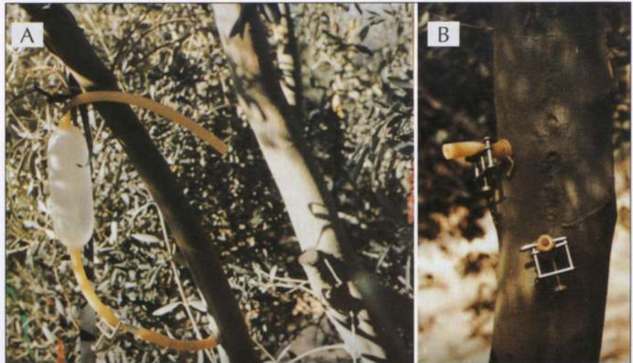
PHOTOGRAPH 38. A low pressure injection system (A) developed for introducing chemicals into the transpiration stream of growing olive trees. After injection the port is sealed off (B).
