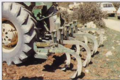
A spring tine cultivator is often used for tilling olive orchards. Vertical tilling is preferable to using a disk harrow.
