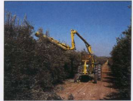
Mechanical harvesting can be applied in intensive orchards. The rotating disks of the pruning machine cut the braches in such a way as to maintain the desired canopy volume.
