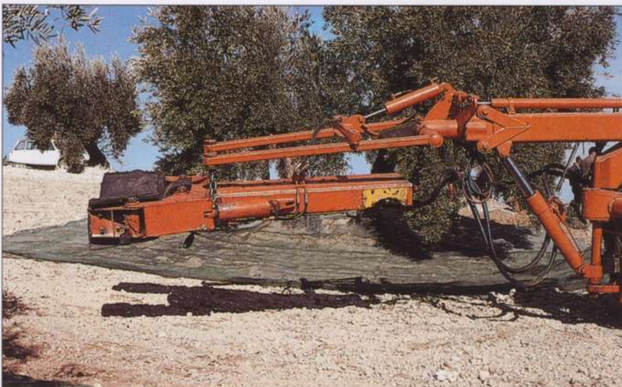
Detail of the multi-directional trunk shaker head used for mechanical harvesting of olives.
