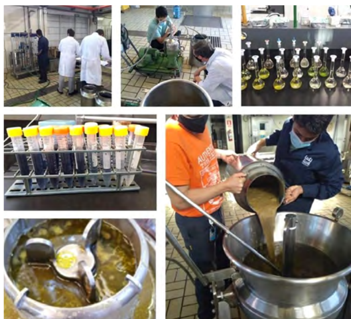
Polyphenols extraction at the pilot plant and quantification in the laboratory
