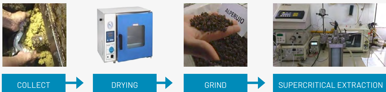
Flowchart showing the process for obtaining antioxidant extracts from solid waste using supercritical fluid technology
