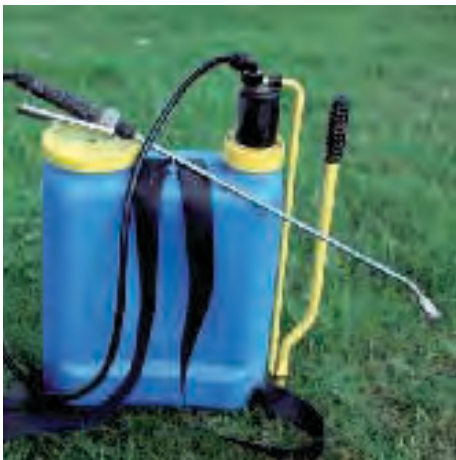
Figure 2. Knapsack sprayer with hand-operated lever.
