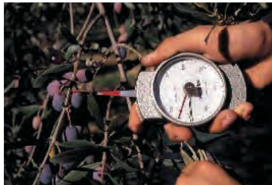
Figure 5. Dynamometer with spiked sensor for determining fruit removal force.
