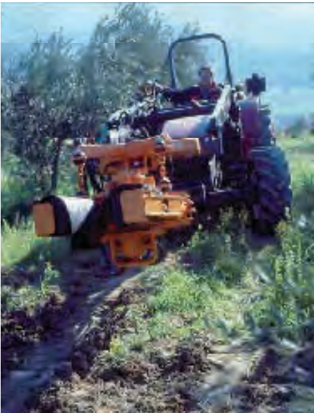
Figure 21. Shaker with two vibrating masses and two engines.
