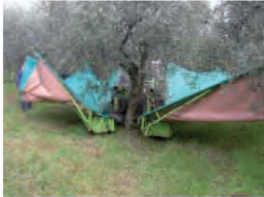
Figure 40. Trunk shaker and wrap-around catching frame make a very efficient combination.
