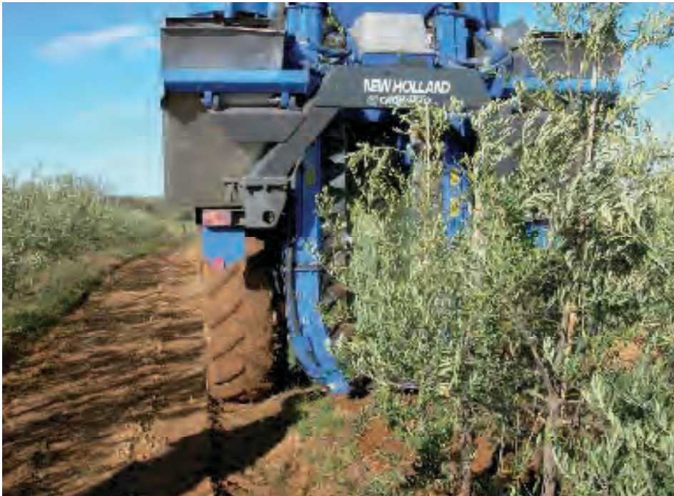
Figure 31. Superintensive orchard with over-the-row harvester.
