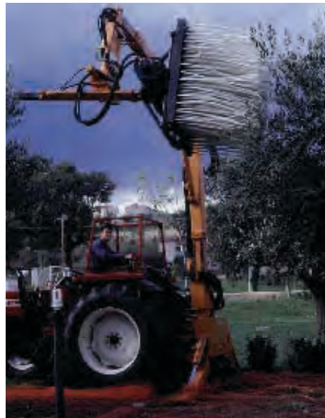
Figure 18. Oscillating rod beater.
