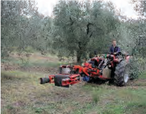
Figure 23. Shaker with a single eccentric mass.
