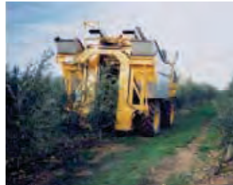
Figure 25. Shaker featuring larger shaker cage.
