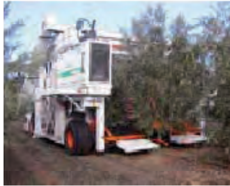
Figure 27. Giant over-the-row harvester.
