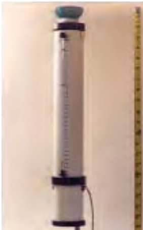
Figure 2. Atmometer (from Altenhofen, 1985)
