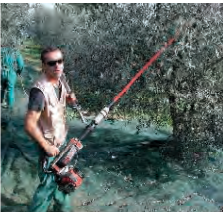
Figure 17. Mechanical hand-carried shaker.
